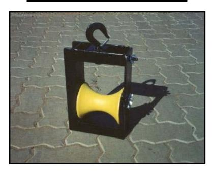
Aerial rollers are used for stringing bundled insulated conductors up to 120 mm outside diameter in overhead distribution schemes. Rollers are suspended from a 750kg safety hook. Cable is fed through a side opening lockable latch. Rollers are available in polyurethane or alluminium. Aerial rollers are manufactured on order only. A lead time of 2 weeks is applicable subject to quantities and roller selection.
