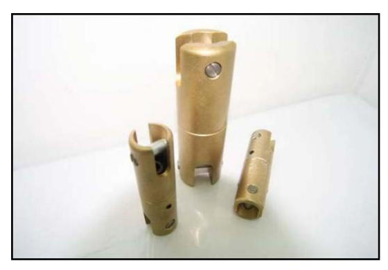
Swivels are essential for effective cable pulling operations. The swivels are fitted with thrust bearings to prevent build up of twist in the cable and rope. Swivels are manufactured from steel with an electro plated finish.
