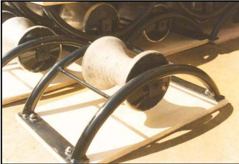
The CR3 cable laying roller is a heavy-duty roller with the frame manufactured from tubular steel fixed on a wooden base. The roller is cast aluminium complete with maintenance free vesconite bushes fitted to the sides. This roller is used for heavy duty laying on sand, trenches or soft ground. CR3 rollers are manufactured on order only. A standard lead time of 3 weeks from receipt of order is applicable.
